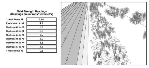
Figure 16. Field measurements collected by Smith-Root Inc. of voltage variation being emitted between electrodes on the electric barrier in Milford Creek Iowa, USA on May 4th, 2022. Stray voltage was also measured 1 meter above and below the barrier.
