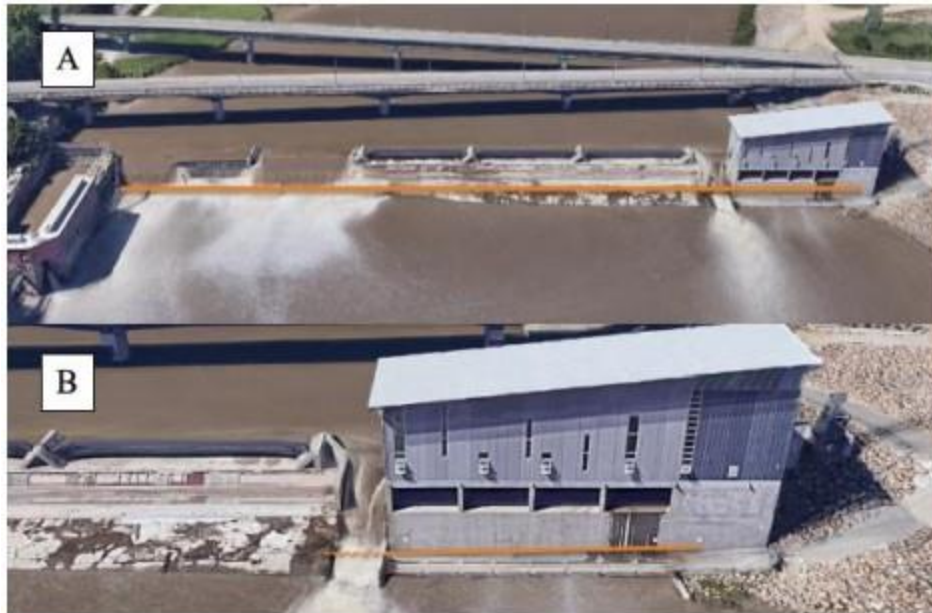
Figure 2: Satellite imagery of Bowersock Dam. Orange lines represent (A) the width of the entire dam and the extent for the acoustic deterrent system described in scenario 1, and (B) the width of the powerhouse (solid line) and Obermeyer gate (dotted line) and the extent of the acoustic deterrent system described in scenario 2. Images were captured using Google Earth®.
