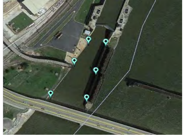
Figure 2. Stationary receiver array around Lock and Dam 19 and the USFWS VPS array in the downstream approach of the lock chamber.
